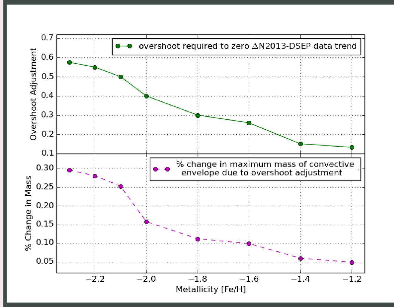
The top panel shows the overshoot adjustment required by DSEP's calculations to zero the model's predictions with N2013's observations. This demonstrates that, in order for DSEP to predict accurately the magnitudes of the most metal-poor stars, overshoot values of up to 0.6 scale heights *H* may be required.
